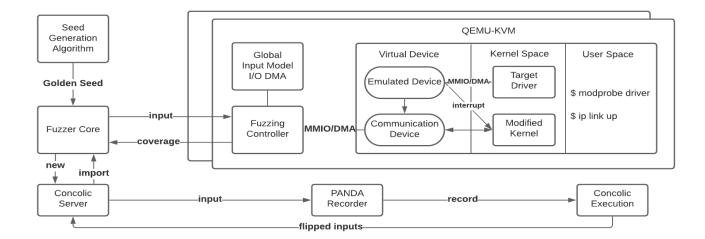
Figure 1: OS-peripheral boundary fuzzing with Drifuzz: our golden seed generation algorithm creates good initial inputs to overcome difficult checks during driver initialization. These seeds are then used as a starting point for a hypervisor-based concolic fuzzer that tests deeper code in the driver by repeatedly restoring a VM snapshot, initializing the driver, and feeding fuzzer-generated inputs via a virtual peripheral.
